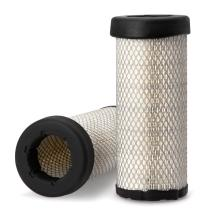
Height251.50 mmLargest ID59.50 mmLargest OD112.00 mmOutside Seal Diameter112.00 mm
