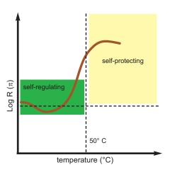
The initial short-term current draw will be approx. 15 Amps and will reduce to 1.5 Amps during regular operation. There is no risk of overheating as the electrical resistance will increase dramatically (ratio of 1 to 10,000) above the designed maximum temperature of 50°C and no current will be drawn.
