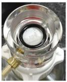
Figure 4. O-ring placement
