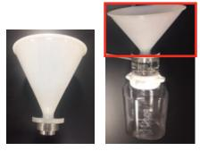
Figure 5. Connecting the funnel assembly
