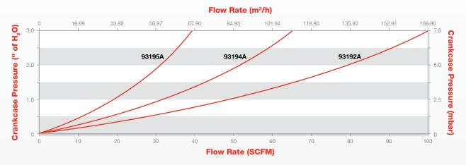
Sizing and installation of the EcoVent Recirculator require an initial maximum pressure of 0" to 0.3"  $\rm H_2O$  (0-0.75 mbar) at engine load with a clean element.
