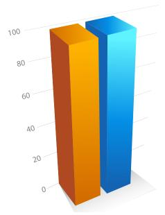
+99% water removal efficiency, tested with ULSD (SAE J1839)
