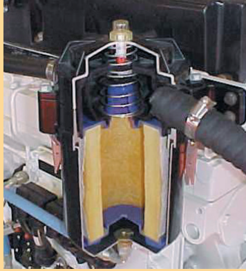
Cummins QSM11 marine engine with CCV cutaway
