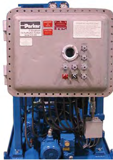
NEMA 7 Explosion Proof
