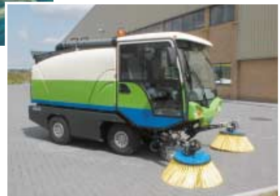
The machine pictured is the "Compact 40" precinct sweeper from the Johnston Compact range of self propelled suction sweepers. Photograph courtesy of Johnston Engineering Ltd.
