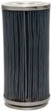
Field Test Sample Retained shape, did not collapse or distort
