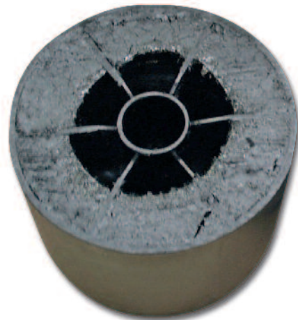
Sectioned Rotor with Contaminant
