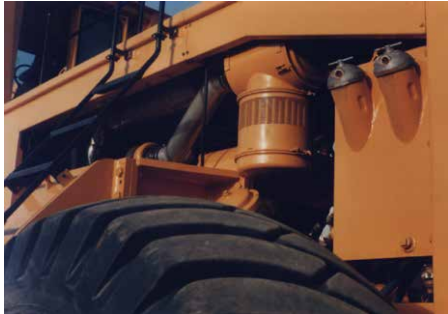
This STG Donaclone, mounted on a large mining machine, is protecting the engine from harmful dirt in this severe dust environment.
