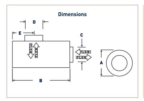
The original ECO Series product, the ECOLITE is still the only air filter in the industry that you can flow air in either direction. This allows a variety of installation options with the same part number replacement filter.
