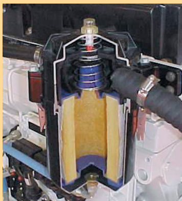
Cummins QSM11 marine engine with CCV cutaway
