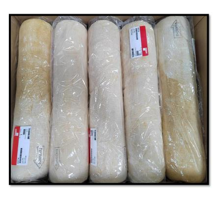
The marks that are mentioned are of visual appearance and will not affect functionally, these are originated by the drying process.
