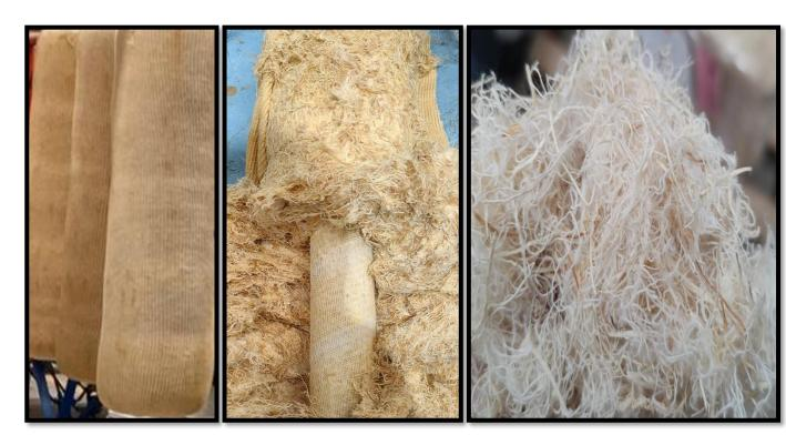
This type of filters have a chemical process which is placed after the assembly process and then a drying process, it will have a rigid appearance to the touch by the immersion process that takes the filter and then is dried to have a humidity less than 10% this condition of rigidity to the touch does not affect its functionality.
