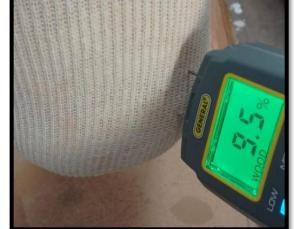
Humidity control was implemented with a hygrometer instrument with 100% verification, which for this type of filter should be less than 10% humidity to prevent possible contaminants.
